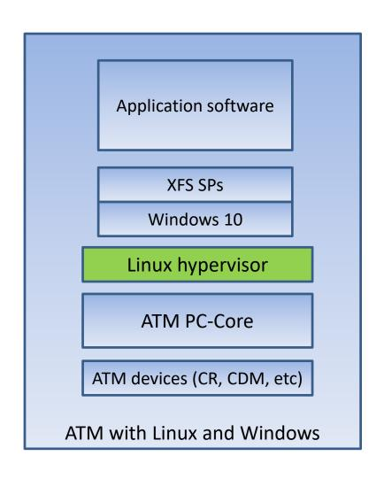
The solution involves inserting a Linux Hypervisor between Windows 10 and the hardware.
